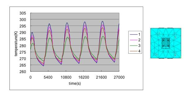
Fig.4 Variations of the satellite temperature.
