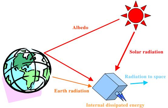
Fig.1 Satellite thermal environment.
