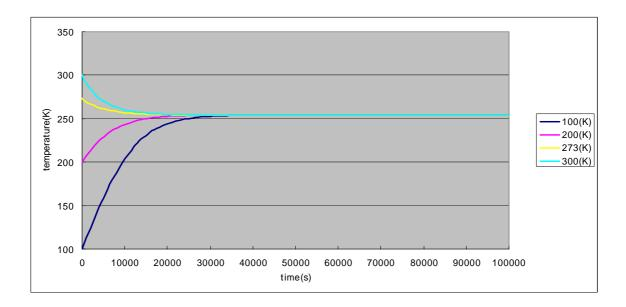
Fig.3 Temperature of the satellite vs. time (ANSYS).
