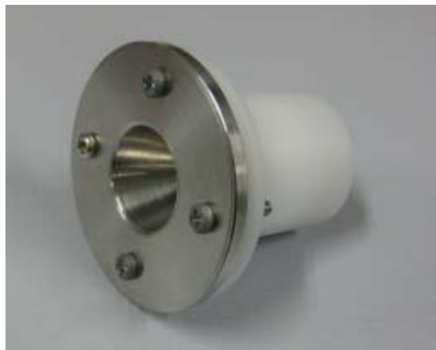
Fig.10 Photo of electrothermal PPT onboard PROITERES.
