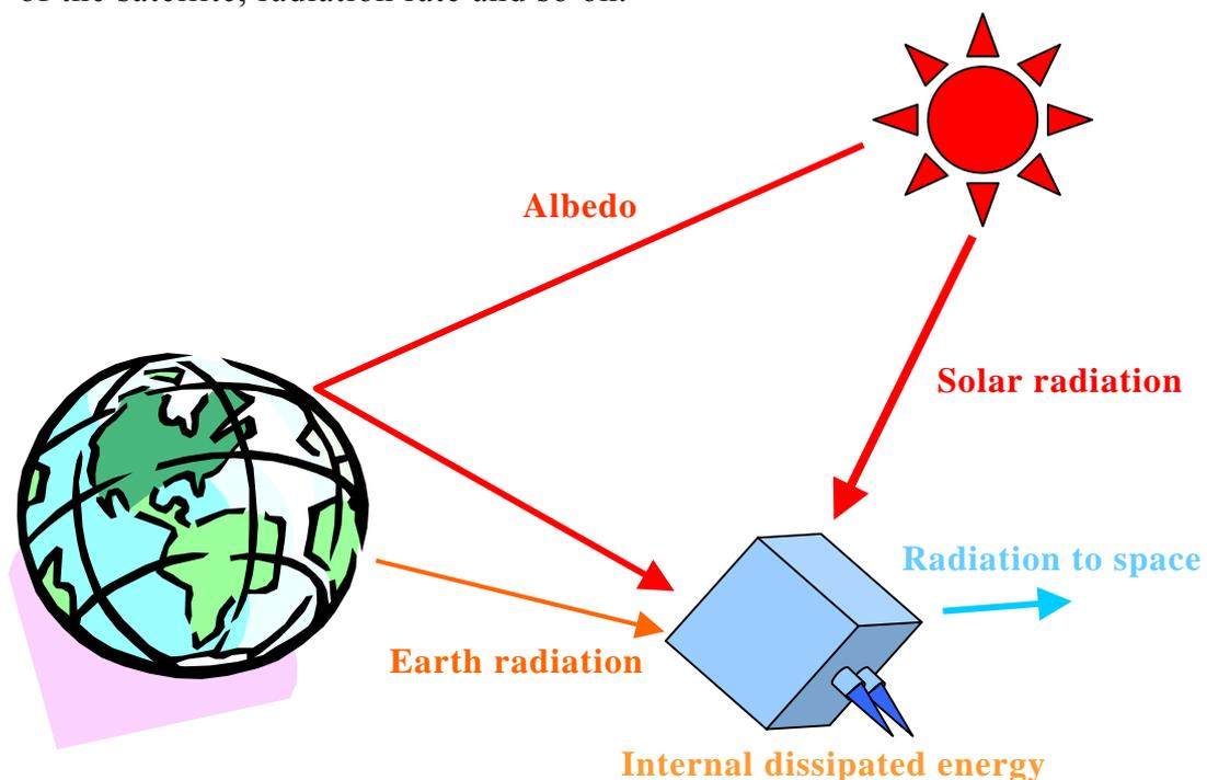
**Fig.1 Satellite thermal environment.**
