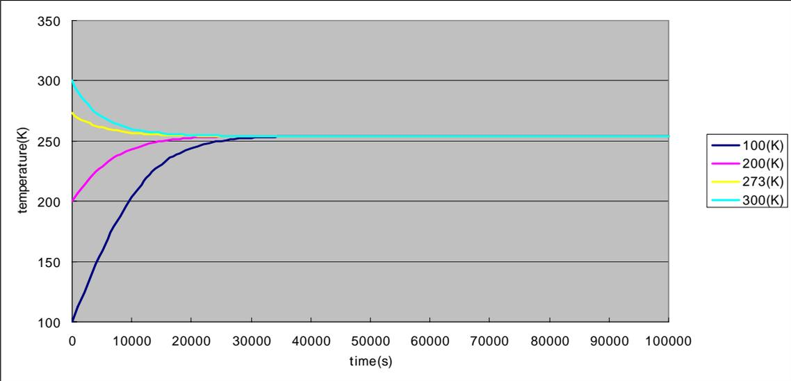
**Fig.3 Temperature of the satellite vs. time (ANSYS).**
