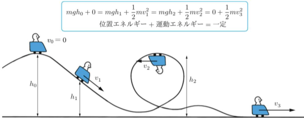
**Figure 8:** Jet coaster does not have its engine. The initial potential energy decides its later velocity.
