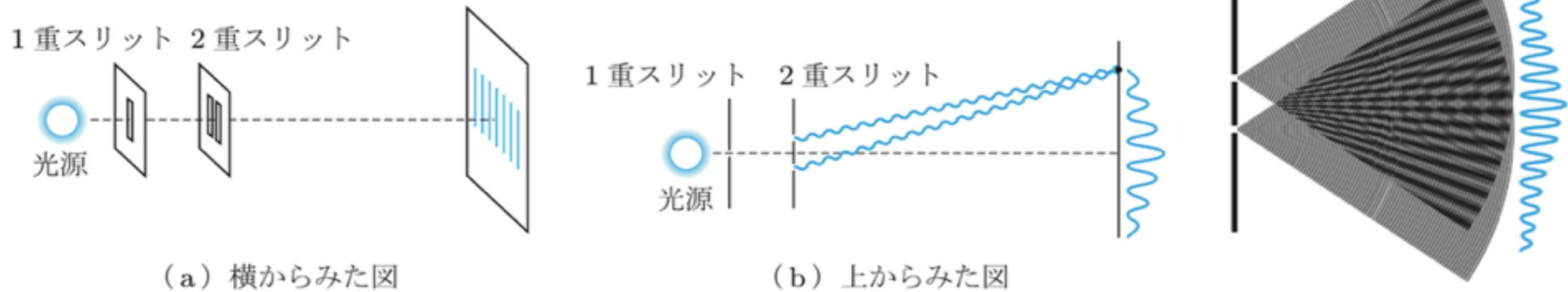
**Figure 15:** Double-slit experiment of light.
