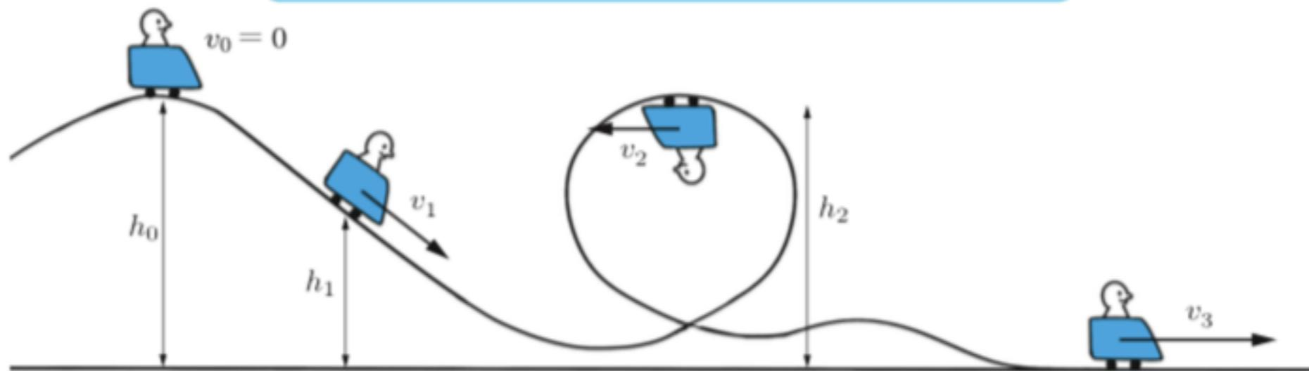
**Figure 8:** Jet coaster does not have its engine. The initial potential energy decides its later velocity.
