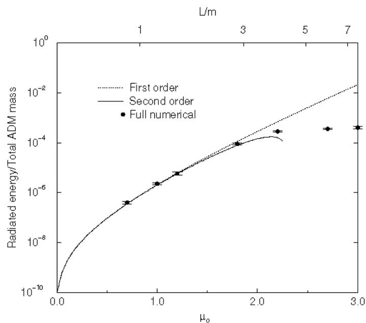
Fig. 3. The radiated energy in a collision of two momentarily-stationary black holes (the Misner problem) compared with the results of full numerical simulations of the NCSA/Potsdam/WashU group. We see that the approximation works well for black holes that are closer than about six times the mass of each hole.
