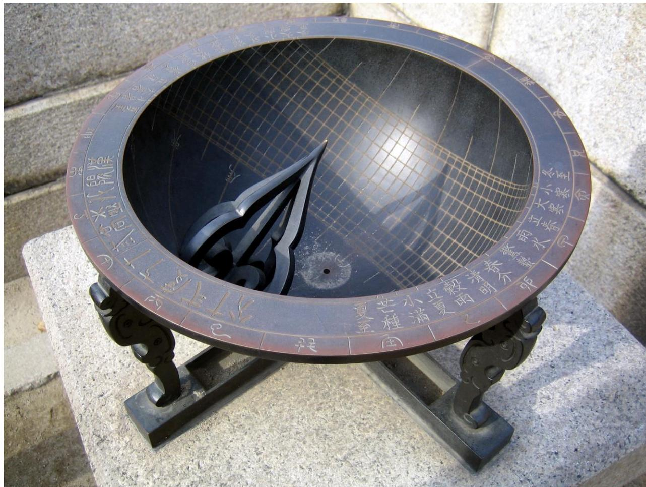
It becomes sundial during the daytime by using the diurnal motion of the Sun, and star-clock during the night time by using the diurnal motion of the Polaris
