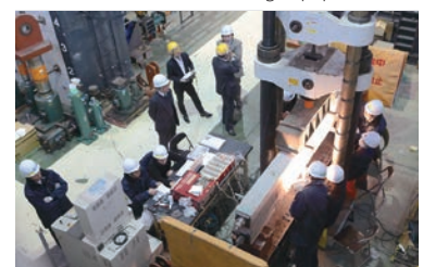
Loading test of prestressed concrete beam
