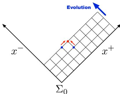
**Figure 3.** Numerical grid structure. Initial data are given on null hypersurfaces  $\Sigma_{\pm}$  ( $x^{\mp} = 0$ ,  $x^{\pm} > 0$ ) and their intersection  $S$ .
