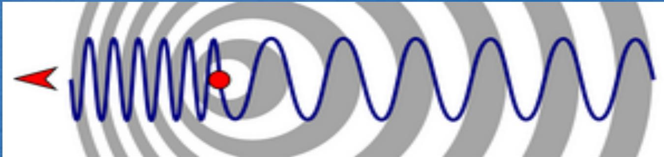
$$f_N = \frac{c + v_{source}}{c - v_{obs}} f_{source}$$
