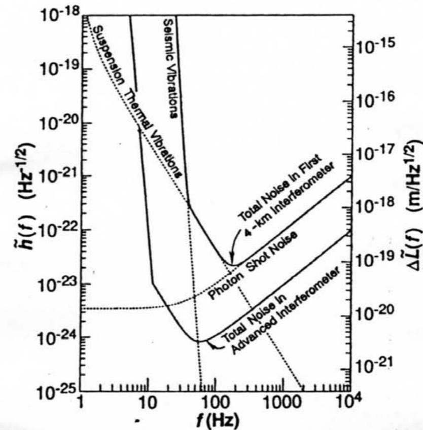
**Fig. 7.** The expected total noise in each of LIGO's first 4-km interferometers (upper solid curve) and in a more advanced interferometer (lower solid curve). The dashed curves show various contributions to the first interferometer's noise.
