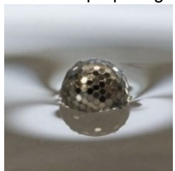
Fig. 1 Polyhedral LM prepared by rolling method
