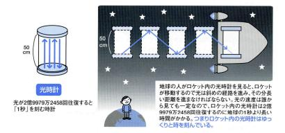
Figure 18: (Left) A light-clock. (Right) When the clock is in a rocket at large speed, a light-ray has to move longer distance for traveling between two mirrors, which means one second in a rocket is longer than that on the Earth.
