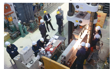
Loading test of prestressed concrete beam
