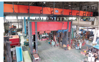
10,000kN Vertical loading equipment
